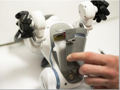
• There are three small hex screws connecting the battery to CHiP. Remove all screws with a hex screwdriver and remove battery casing.
