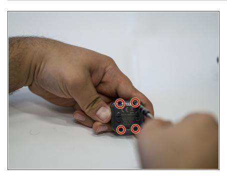
Remove the four screws in the back of the watch using a Phillips #0 screwdriver.
