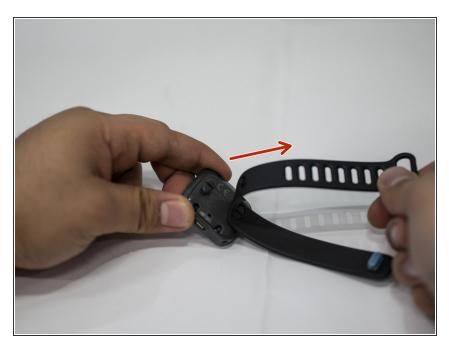
Remove the wrist strap by gently pulling the band off of the plastic pegs on the back of the watch.
