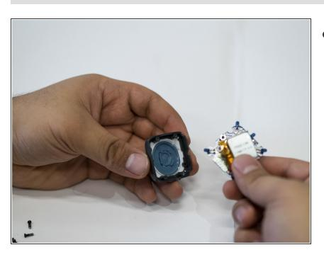
Pull the battery and motherboard component out.
