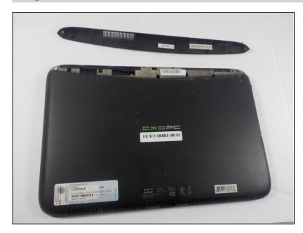
Turn the PC on its back with the screen facing down and pull on the piece of plastic shown in the image. Use your fingernails to prod into the depression where the two plastic covers meet.
