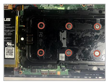
Use a Phillips #000 screwdriver to remove the six 0.6mm screws that secure the dock station case to the motherboard.
