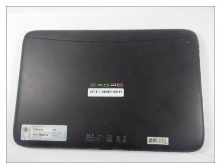
Turn the PC on its back with the screen facing down and pull on the piece of plastic shown in the image. Use your fingernails to prod into the depression where the two plastic covers meet.
