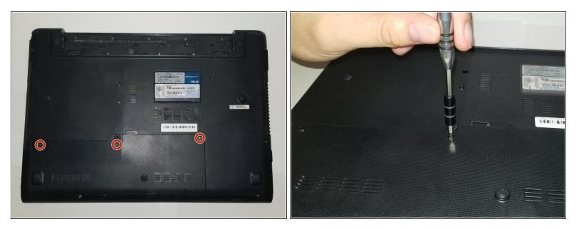
• Using a Phillips #00 screwdriver, remove the screws.
