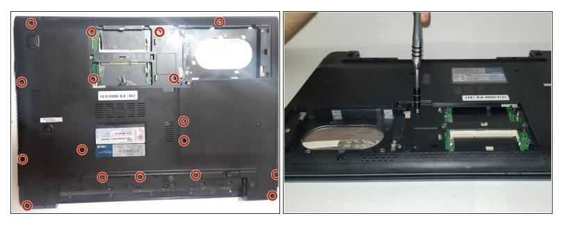
• Using a Phillips #00 screwdriver, remove the screws.
