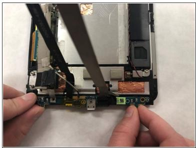
• Remove lower flex cable and LCD flex cable. They are attached and will be removed as one piece.
