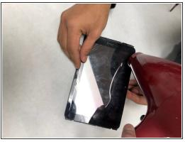
Release the adhesive around the edges of the screen with a safe open pry tool. Continue to reheat the adhesive as needed.
