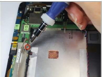
Remove the four 2.5mm Torx #5 screws that run along the motherboard's rim.
