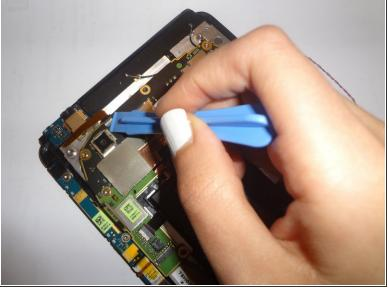
Remove the cable along the headphone in the same way the lower cables were removed.
