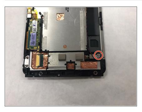
Remove the single 2.5mm Torx T5 screw.
