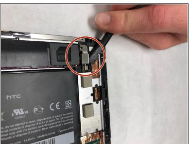
Lift casing away from vibrate motor.
