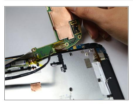
Grip the motherboard by its edges and pull it out.
