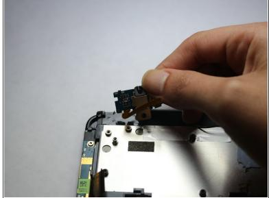
Remove the single 2.5mm Torx T5 screw.
