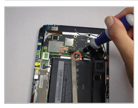
Remove the single 2.5mm Torx T5 screw holding the battery down along the top side.
