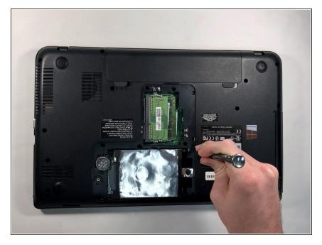
Remove the 4mm Phillips #1 screw on the side of the now exposed area.
