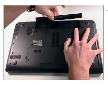
Lift the battery upward with your fingers out of the battery compartment.
