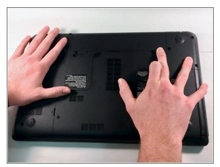
Press down with your fingers while also applying a sliding motion on the latch buttons near the battery on the underside of your laptop.
