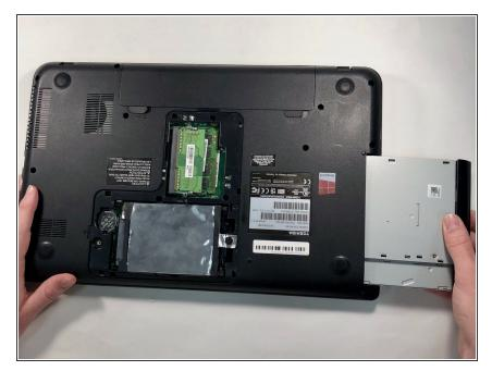
Remove the disc drive from the device.
