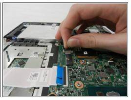
Disconnect the following cables that connect to the motherboard: hard drive cable and touchpad cable.
