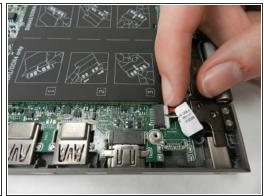
Disconnect the following cables that connect to the motherboard: the Touchscreen, Display, and the speaker cable.
