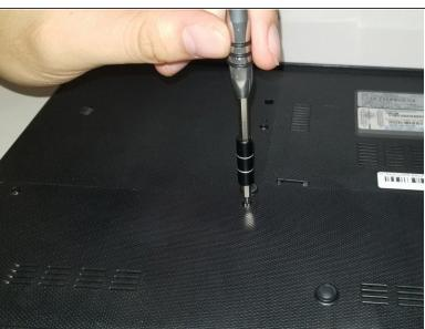
Using a Phillips #00 screwdriver, remove the screws.
