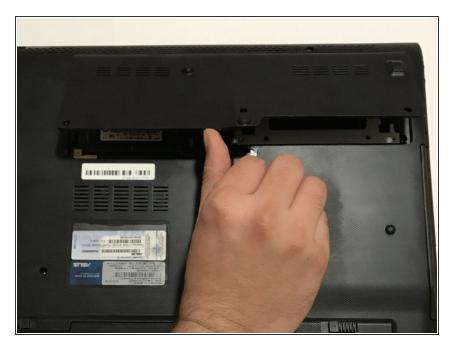
Lift backplate and remove from the case.
