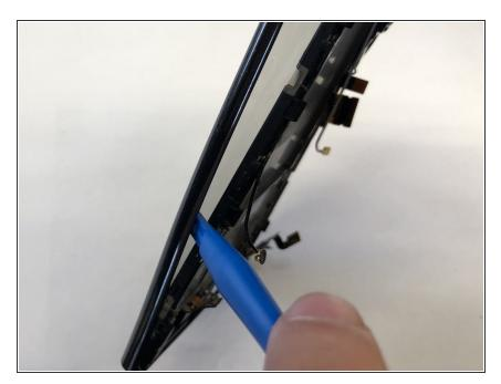
Carefully use the plastic opening tool to pry the screen protector from the display and motherboard.
