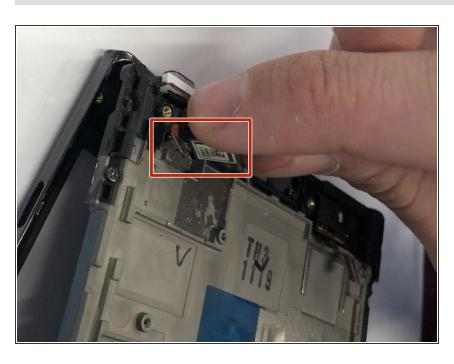
Carefully pull the ribbon cable upward and away from the front screen display.
