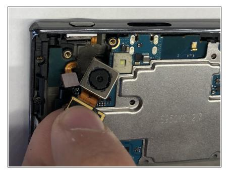
Using the ribbon beneath the camera lift it upwards and pull the camera out.
