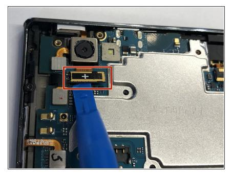
Carefully use the plastic opening tool to pry the ribbon cable below the camera itself from the motherboard.
