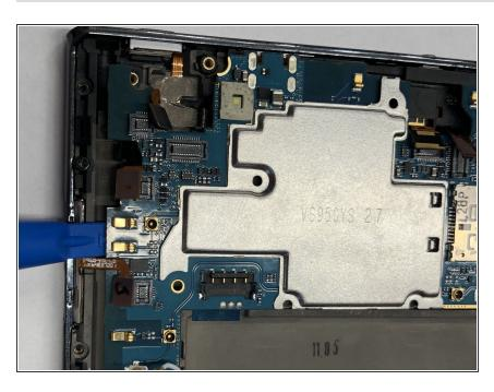
Carefully use the plastic opening tool to pry the motherboard from the front screen.
