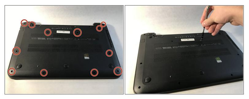
Use JIS #1 screwdriver to remove the eleven 6 mm screws.
