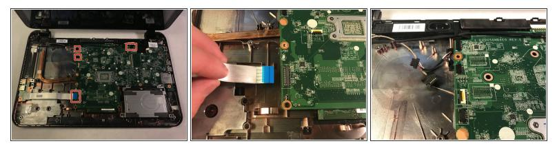
Disconnect the cables to the motherboard.
