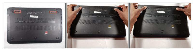
Push both buttons towards one another simultaneously. The battery slightly pops out.
