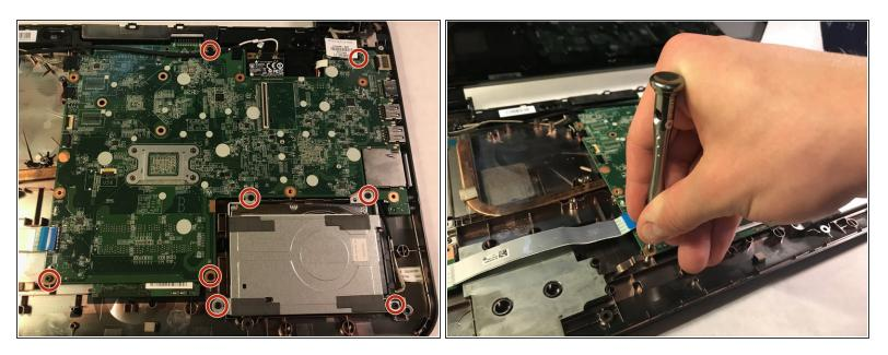
• Remove the eight 5 mm screws with the JIS #1 screwdriver.
