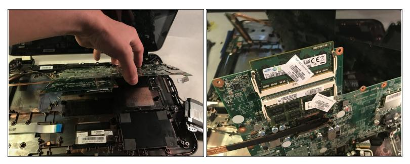
• Lift up the motherboard from the bottom side of the device.
