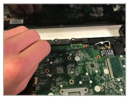
Unclip the WLAN cable out of its place to allow the motherboard room to move.
