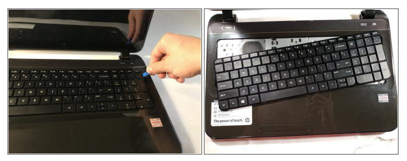
• Using a plastic opening tool, release the keyboard clips.
