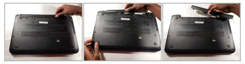
Pull out the battery from the device's battery slot.
