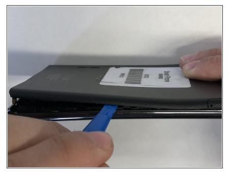
Carefully use the plastic opening tool to pry the back panel of the phone from the front screen. This will expose the battery and other parts.
