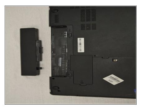
Remove the battery from the device.
