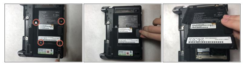
Remove back cover of the device by unscrewing the four 7mm screws with a Phillips #0 screwdriver.
