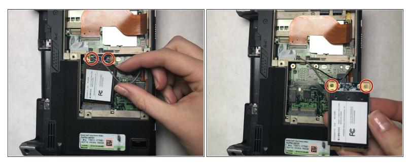
Detach the two antenna cables connected to the wireless LAN card by gently pulling them out of place.
