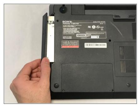
(i) Slide in new CD drive and repeat steps 2 and 1 in reverse to screw the new drive down.
