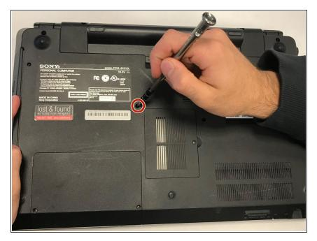
Remove the second of the two screws located at the marker in the photo.
