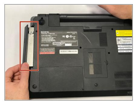
Grab and slide out the tray from the side of the laptop after both screws have been removed.
