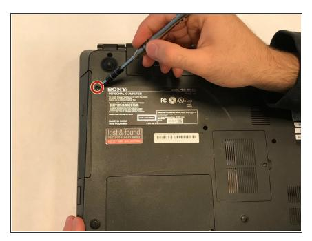
Remove the first of two screws located at the marker in the photo.
