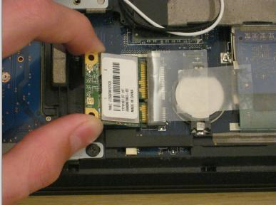
Just like RAM, hold the WLAN card by the edges and pull it out at an angle.
