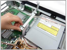
Using your fingers, gently remove the metal pieces on each side of the cartridge and carefully place them aside.
