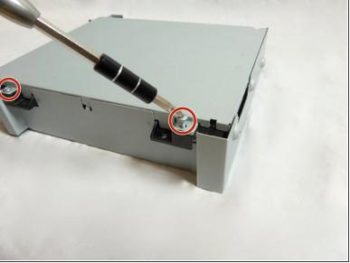
• Flip the cartridge over to the bare side with no stickers. Remove four 10mm Phillips screws from each corner.
