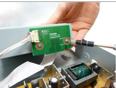
Gently lift the cartridge. Remove two 4mm Phillips screws from the green circuit board.
