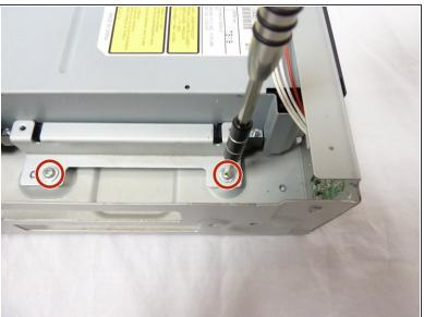
Remove the remaining four 6mm Phillips screws.
