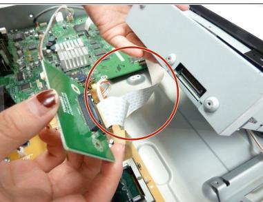
• Using your fingers, pull off the green circuit board from the cartridge and carefully place it down.
