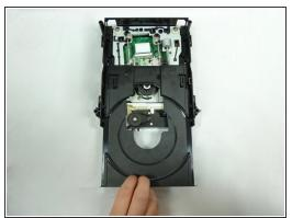
Slide out the disc tray. If it's stuck, turn the white gear to the right to release the tray.
