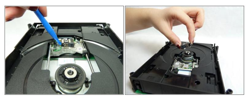
• Using a prying tool, wedge the edge of the tool underneath the end of the optical lens closest to the green circuit board. Gently push down to pop off the optical lens.
