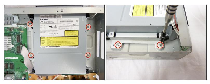
• Remove the remaining four 6mm Phillips screws.
