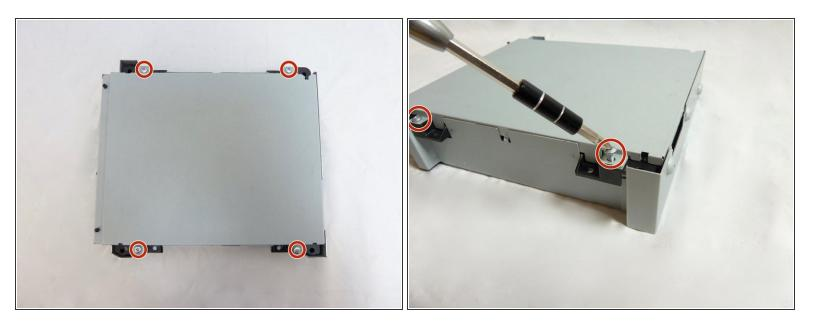
• Flip the cartridge over to the bare side with no stickers. Remove four 10mm Phillips screws from each corner.
