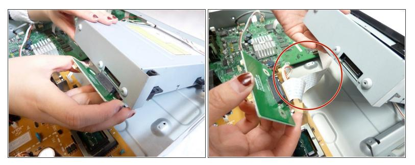
• Using your fingers, pull off the green circuit board from the cartridge and carefully place it down.
