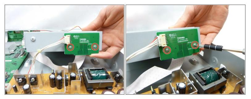
• Gently lift the cartridge. Remove two 4mm Phillips screws from the green circuit board.
