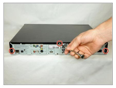
Remove the three 6mm Phillips head screws on the back of the DVD player with a Phillips #1 screwdriver.
