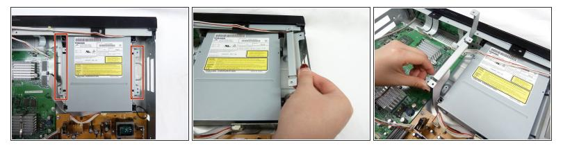
Using your fingers, gently remove the metal pieces on each side of the cartridge and carefully place them aside.
