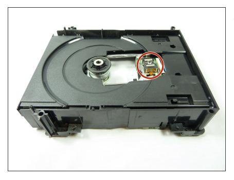
• The optical lens will be resting aside the small green circuit board.
