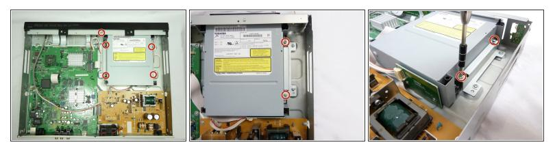
• Remove five 6mm Phillips screws with a Phillips #2 screwdriver.
