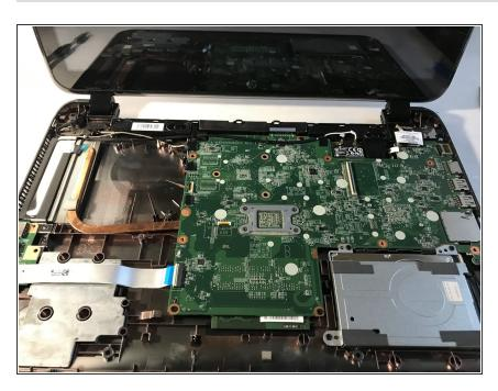
Carefully remove the fan from its slot.
