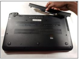
Pull out the battery from the device's battery slot.
