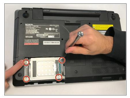
Remove the screws keeping the hard drive in place.
