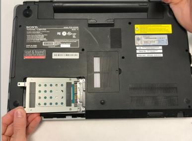
Lift the hard drive carefully and replace with a new one.
