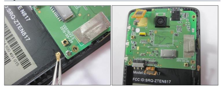
• Disconnect the coaxial connector in the bottom right corner of the motherboard.
