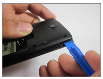
Carefully pry open the back panel with the plastic opening tool.
