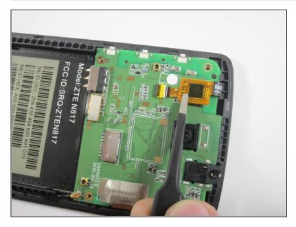
Use a pair of <u>tweezers</u> to gently disconnect the ribbon cable connector from its socket.
