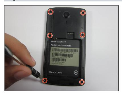
Use the JIS #000 screwdriver to remove the six 3.0mm screws placed in the back of the ZTE Quest.
