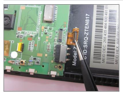
Unplug the flat-top connector by using a pair of tweezers to pry up each side before removing the connector from its socket.
