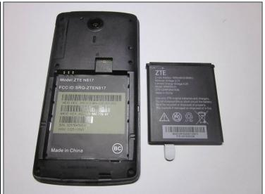
Use the ribbon to remove the exposed battery.
