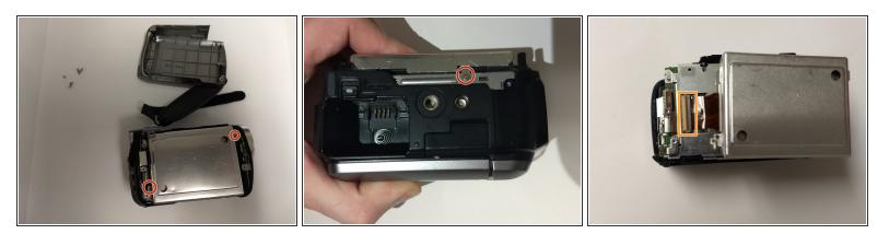
• Remove the three screws highlighted in the pictures shown.
