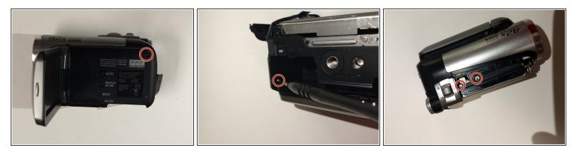
Remove indicated screws to release back panel.
