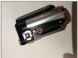
Remove indicated screws to release back panel.
