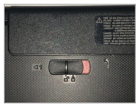
Slide the manual battery latch to the unlock position, so that the red is showing.
