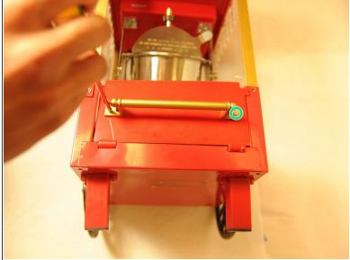
With the Phillips #1 screwdriver, unscrew and remove the two, 12mm screws on the outside edges
