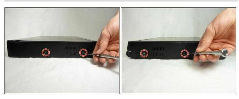
Remove the two 3mm Phillips screws on each side of the DVD player using the Phillips #1 screwdriver.
