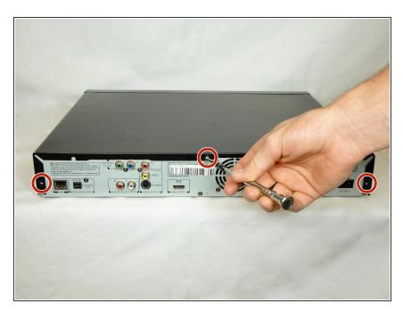
Remove the three 6mm Phillips head screws on the back of the DVD player with a Phillips #1 screwdriver.
