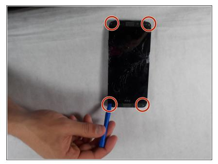
Remove the four 1.2mm screws in the corners to release the front of the phone from the back, then pry it off with the plastic opening tool.
