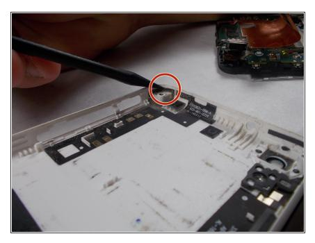
Use a spudger to gently lift one side of the antenna strip up, then pull it off. This needs to be done in all four corners.
