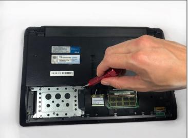
• Remove the four screws with a Phillips #0 screwdriver.
