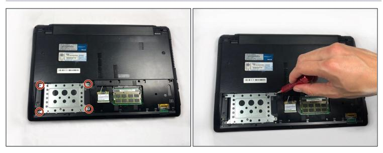
• Remove the four screws with a Phillips #0 screwdriver.
