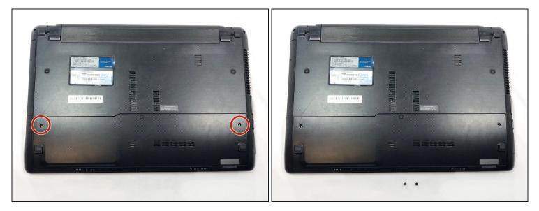
• Use a Phillips #0 screwdriver to remove the two screws circled in picture.
