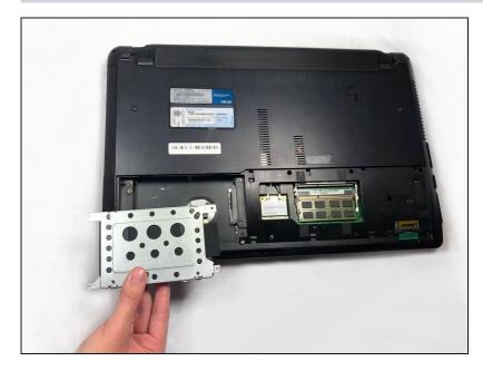
• Remove the hard drive from the device.
