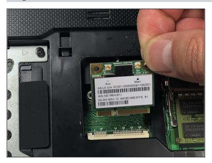
Remove the Wi-Fi card from the device.
