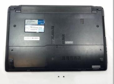
Use a Phillips #0 screwdriver to remove the two screws circled in picture.
