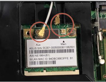
• Remove the two pin connectors from the wifi card.
