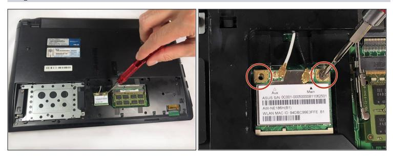
• Remove the two screws using the Phillips #0 screwdriver.
