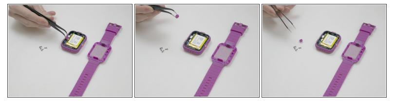
After removing the backplate, lift the master switch up from the circuit board.
