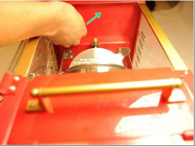
Unscrew the bulb located in the top left corner of the machine in a counterclockwise direction until the bulb is no longer attached. To reassemble your device, follow these instructions in reverse order.
