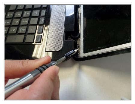
• Using the same screwdriver (Phillips Head #1), unscrew all the screws on both sides of the screen.
