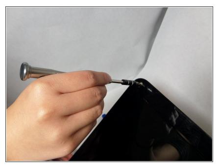
• Unscrew the screws using a Phillips Head #1 screwdriver; there should be four in total, one on each corner.
