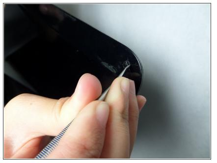
Locate the round stickers on each corner of the screen covering the screws. Use a sharp tool, such as a pointy metal spudger or tweezers, to gently remove these stickers.
