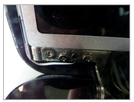
• Locate the two screws at the bottom corners of the screen.
