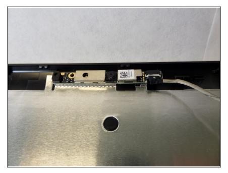
At the top of the computer, there should be a cable still wired to the detached screen. Gently pull the head of the cable away from its connector until the cable dislodges.
