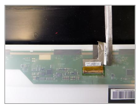
At the back of the screen, there will be one more connector at the bottom. Remove the tape to disconnect this wire.
