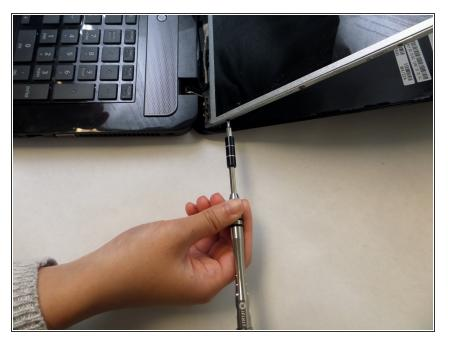
Find and unscrew the six screws (3 on each side) on the sides of the screen. Be careful while unscrewing the last few screws as the screen will still be attached to the computer in two different places and may fall out of its casing.
