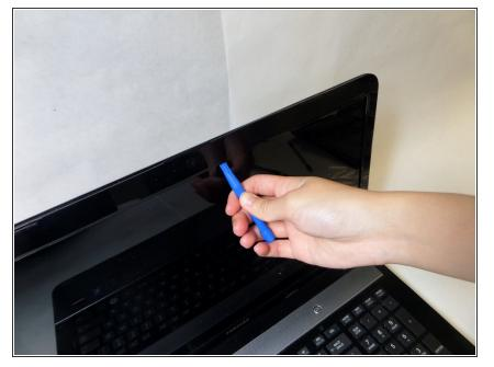
Take the opening tool and gently place it under the plastic framing the screen. Gently slip the opening tool between the plastic frame and the screen, until a change in pressure is felt, the feeling of the plastic clasps dislodging.
