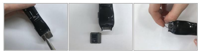
• Remove the screws, then gently lift off the blade. A small piece of plastic should come off with the blade. There will be a spring revealed from under the blade, remove this as well.
