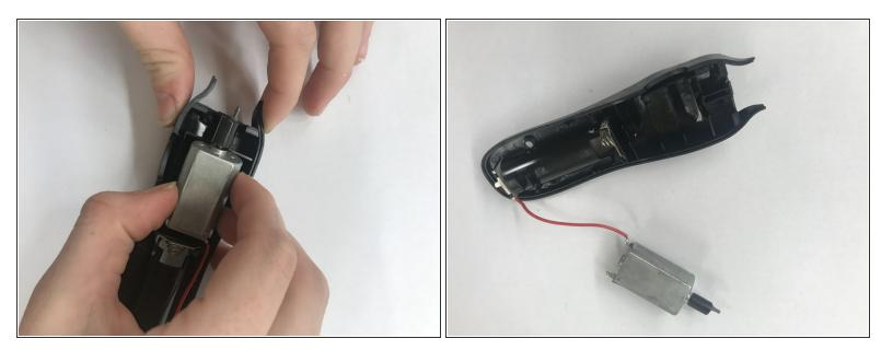
• Finally, remove the motor from the black plastic cover. If desired, this motor can be de-soldered from the red wire and re-purposed.
