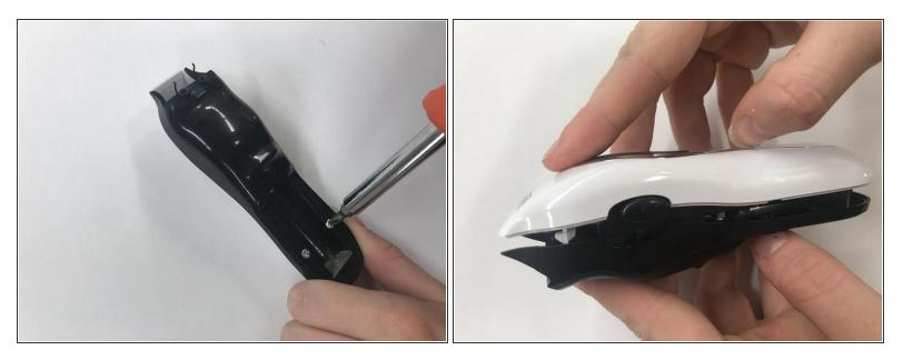
• Remove the screws from the sides of the battery compartment. Then, gently separate the two halves of the plastic cover.
