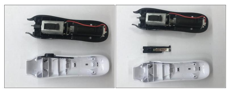
Lay both halves of the trimmer out, and remove the switch from the inside of the white plastic cover.
