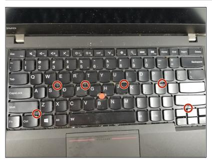
Use a Phillips #00 screwdrivers to remove the six screws holding in the keyboard.
