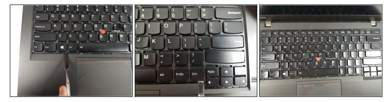
• Use the metal spudger to press the keyboard plate forward towards the display
