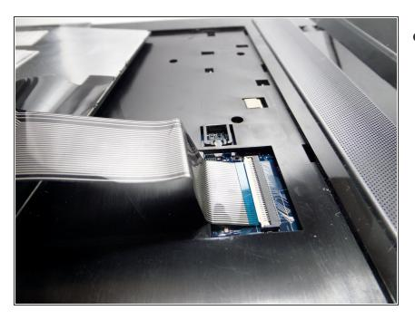
Find the ribbon cable that connects the keyboard to the computer.
