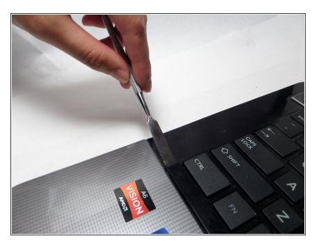
Starting on either side, use a metal spudger to pry out the long, narrow plastic covering at the bottom of the keyboard.
