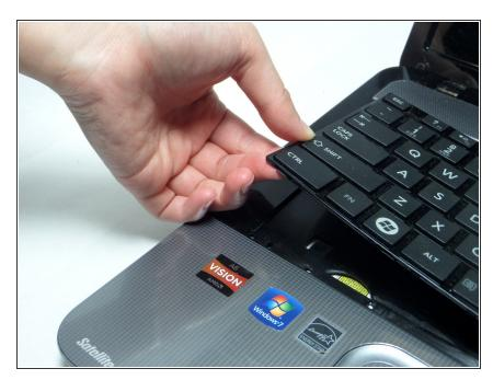
Using your hands, gently lift the keyboard out of the computer. The keyboard will still be attached to the computer so be careful not to pull too hard.
