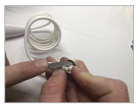
Using an o-ring removal tool or a small flattip screwdriver carefully remove o-ring from pressure pump housing by gently prying the o-ring over the lip of the housing.
