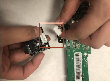
To detach the cables grab the internal power adapter in one hand and with the other grab the base of the wires and firmly pull them straight out from the device. To reassemble your device, follow these instructions in reverse order.
