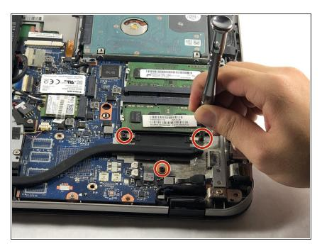
Remove the three 5 mm screws using a Phillips #1 screwdriver.
