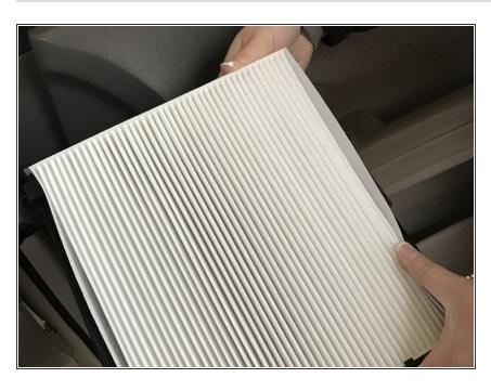
Place the new air filter in the square and push the four corners to lock it into place.
