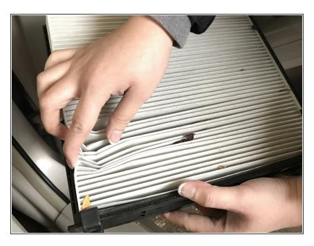
Push the air filter in the four corners to release the old one.
