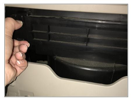
Once the glove box is loose, locate latches, on the left and right top and bottom corners, and pinch together, at the same time, to free the air filter.
