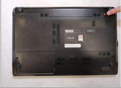
Pull the latch to the right of the battery to the right.
