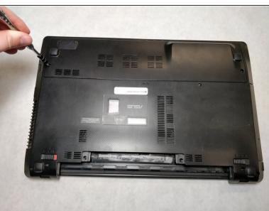
Using a JIS #00 screwdriver, unscrew the two 5 mm screws on either side of the laptop panel.
