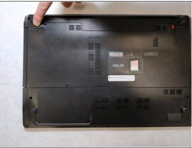
Pull the latch to the left of the battery to the left. Hold the latch open with a finger to prevent it from closing.
