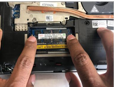
Push apart the two metal clips that hold the RAM in place.
