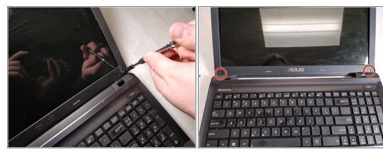
Using a JIS #00 screwdriver, remove the two 5 mm screws that were exposed by the bumpers being removed.
