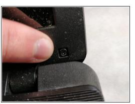
Remove the plugs at the bottom corners to expose the screws beneath.
