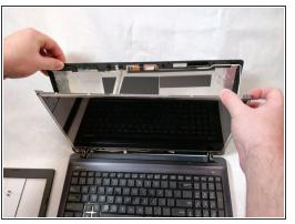
Using a JIS #00 screwdriver, remove the six 5 mm screws from the back plate to screen connections in each of the 4 corners of the screen.
