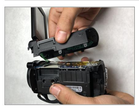
Pull apart the camera into two pieces by pulling the side with the screen away from the main body of the camera.
