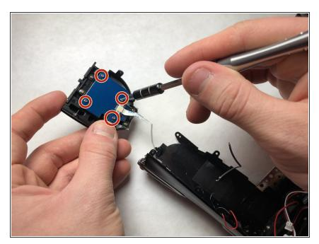
Unscrew all four screws (length 4.13 mm) on the inside of the case with a PH #00 screwdriver.
