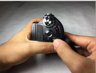
Pull the slider labeled open, on the bottom right, to unlock the battery.
