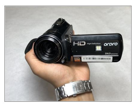
Unfold the screen from the side of the camera.
