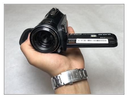
Twist the screen so that the screen is facing downward.
