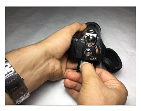
Pull battery out of slot.
