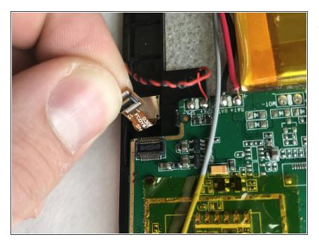
Gently pull the front camera connection out of its socket.
