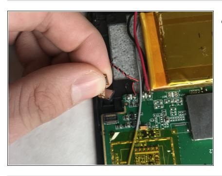
Lift the camera unit from its housing.
