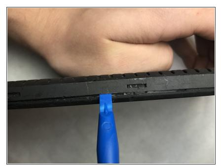
Wedge the plastic opening tool into the seam nearest to the screen surface and begin to pry off the back of the device.
