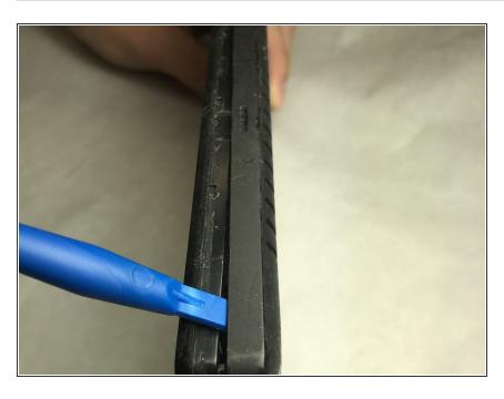
Move the plastic opening tool along the perimeter of the device, loosening the entire back as you go.
