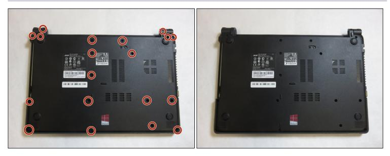
• Remove nineteen screws from the back panel using a Phillips #0 Screwdriver .
