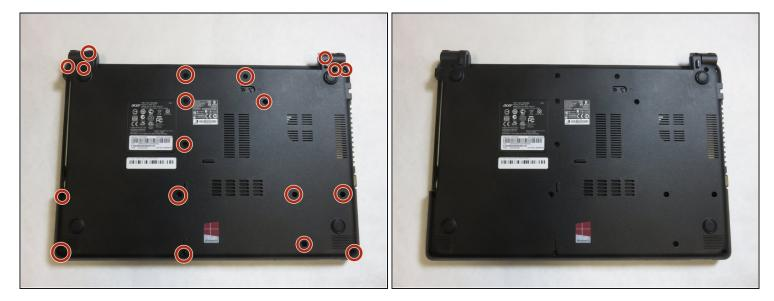
Remove nineteen screws from the back panel using a Phillips #0 Screwdriver.
