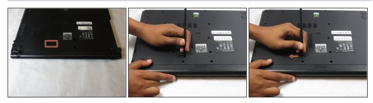
Use your finger or a spuger to pull the battery release switch.
