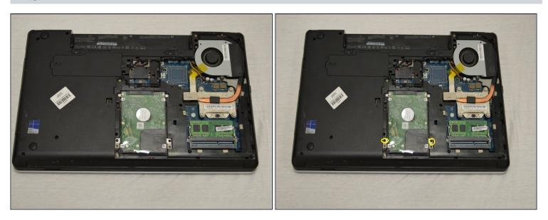
• After back panel is removed, you can remove the two screws at the bottom of the hard drive using the Phillips #000 screwdriver.
