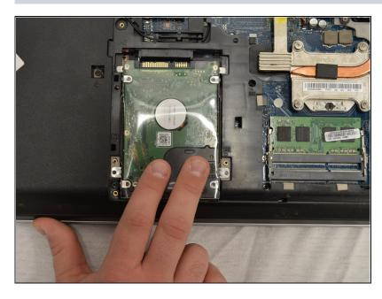
• After screws are removed, slide the hard drive down to disconnect from motherboard and remove it.
