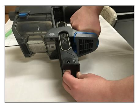
• While squeezing the lever at the bottom of the power pack, pull out the battery pack to remove the battery.
