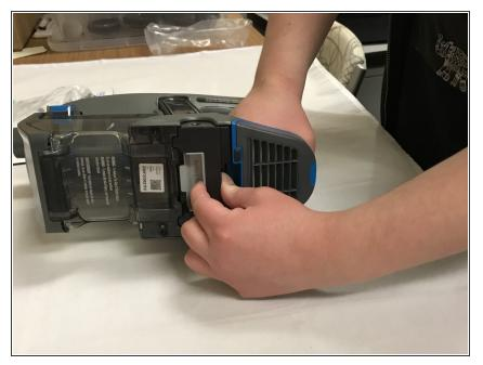
• Squeeze the lever located at the bottom of the lithium power pack labeled "Battery Release".
